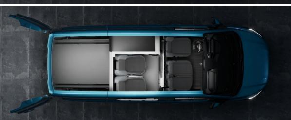
With it's unique bulkhead, the Multicab can offer seating for up to 5 people, and a load length of up to 3450mm (on LWB versions with load-thru)
