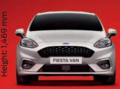
Width: 1,783 mm Width (with mirrors): 1,941 mm Length: 4,065 mm
